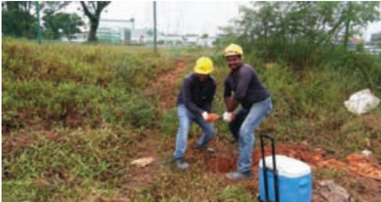
Sampling of shallow soil in Singapore using a Dutch hand auger
